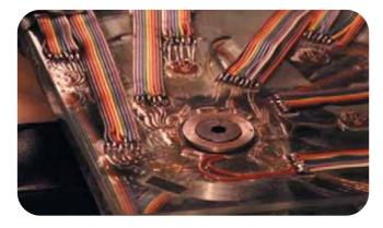
Strain Gauge Testing around Pilkington Planar<sup>™</sup> countersunk hole.
