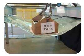
Planar<sup>™</sup> | SentryGlas<sup>®</sup> Plus System Panels undergoing load testing
